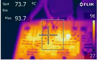
Figure 17 70A Full Load With Fan Cooling
